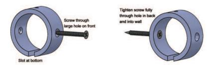
Slide the wall tube through the mounting brackets - the fiber tails will slide through the cut out in the bottom of the brackets,
