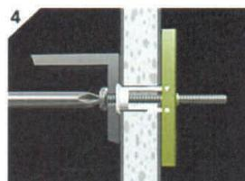
Place item over flange. Insert bolt through item and tighten until flush against item, then stop.
