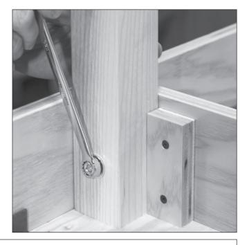
FOR SAFETY PURPOSES, TAKE TIME TO CHECK ALL NUTS TO INSURE THAT THEY ARE SECURELY TIGHTENED AND THAT THE PLATFORM HAS BEEN PROPERLY ASSEMBLED ACCORDING TO THESE INSTRUCTIONS.
