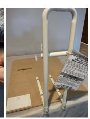
Step 3: Insert Transfer Handle into the base plate (A), pressing in snaps. Ensure that both snaps are fully extended through holes. Secure 7/16" safety nut to fully extended snap bolt with wrench (C.)
