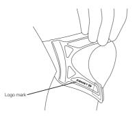
3. Straighten the knee and fasten hook-and-loop fastener A.
