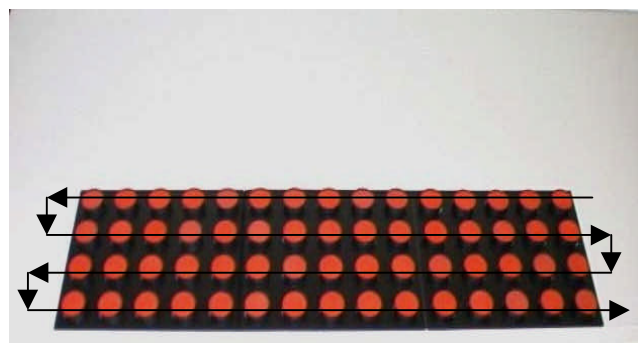
Figure 3 Starting position and sequence of rows with directions of travel for the Turning Test.
