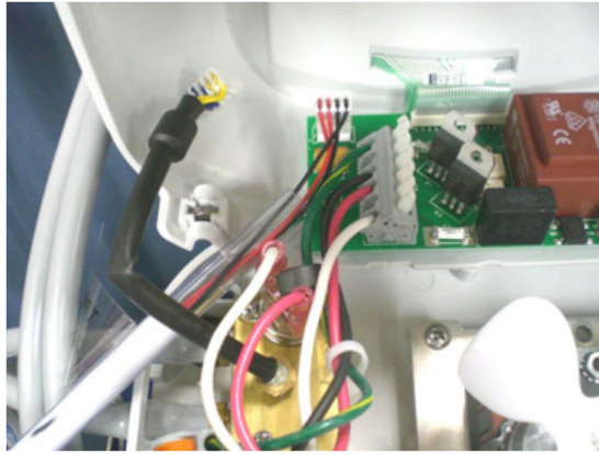
Figure 10: Connection of Test Temperature Sensor
