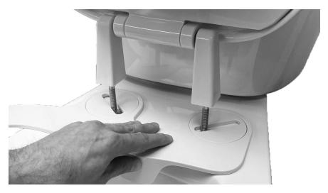
9. While holding down the bidet attachment with one hand, pick up the seat, align the bolts to the mounting holes and push the seat downward through the slots in the circular mounting disks so the bolts enter the seat mounting holes on the toilet. Pushing downward and holding the seat in place, lightly handtighten the Stay•Tite<sup>™</sup> nuts.
