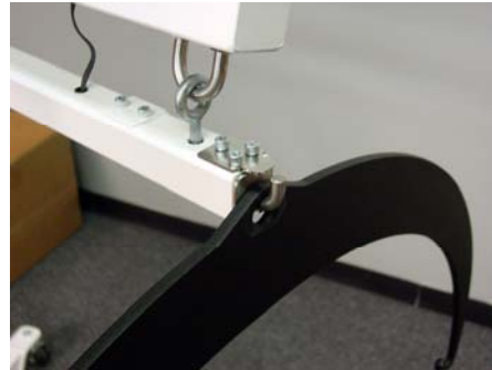
Completely tighten all three retainer plate screws
