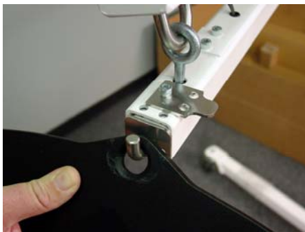
Align hole in Stretcher Hoop with Support Hook
