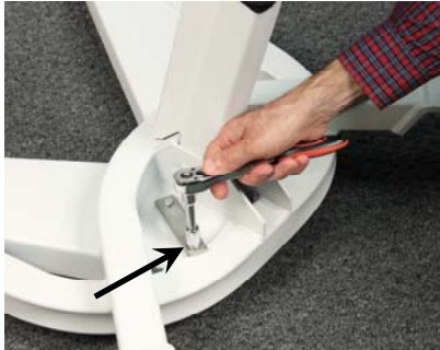
Remove mounting bolt
