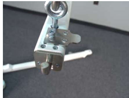
Rotate Hoop Retainer Plate
