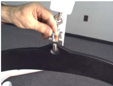
Lift hoop slightly to ease screw installation
