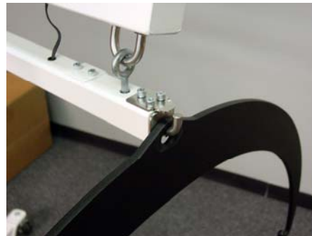
Completely tighten all three retainer plate screws
