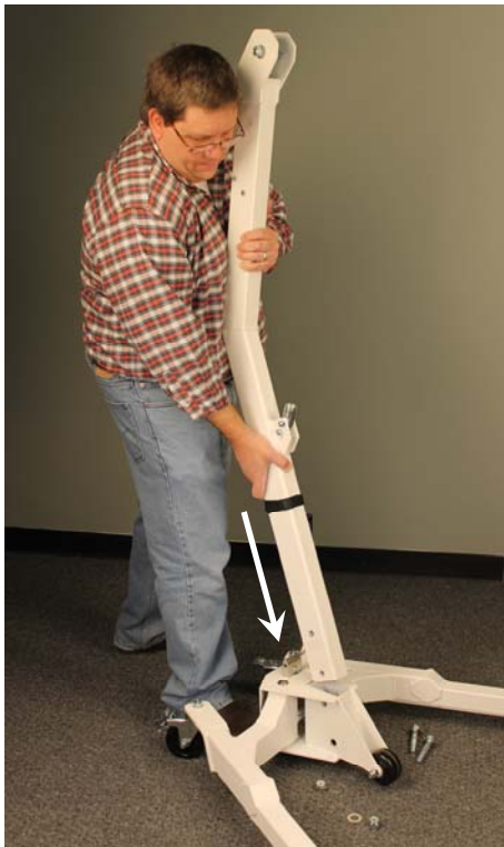
Insert Column at an angle
