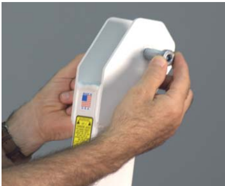
Remove Bolt from Column
