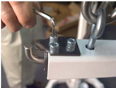
Remove outer 2 Screws Loosen inner Screw
