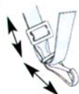
Diagram D While holding on to the loose end, push the bar side and hook up or down the shoulder hook strap to the desired length.
