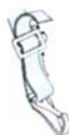
Diagram E Thread the loose end back through the bar slide as shown above (Diagram E)
